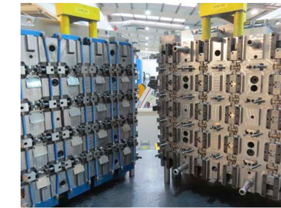
Complex high-precision multi-cavity tooling for the medical sector. Each cavity is individually temperature controlled. This tool runs in a 350-tonne injection moulding machine.
