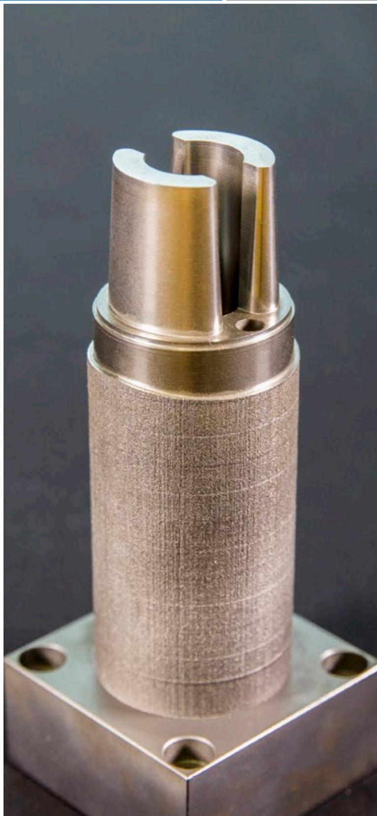
This approach, known as 'conformal cooling', has been around for a long time, but it is rarely used in production applications
